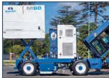
Dumping at any height between 1,1 and 2,3 m.
