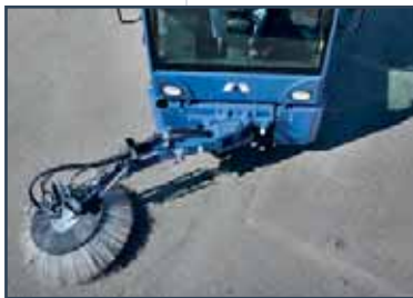
Fully adjustable third front brush that allows to sweep 180° left and right side.
