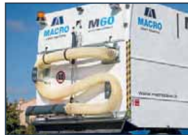
Rear powerful wandering vacuum hose, 6 m length -140 mm diameter.
