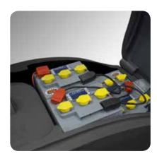
Easy access to battery and vacuum motor compartment, without using tools. Large capacity shock and acid proof polyethilene tanks (88 l) avoid frequent refilling and idle time. 4 x 6V -180 Ah C5 batteries granting continuous working time up to 4-5 hours.
